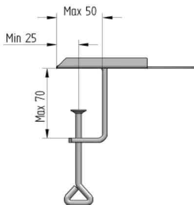
The extraction arms can easily be mounted on a workbench or on a shelf.
