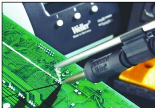
Fume extraction wand attached to soldering iron.
