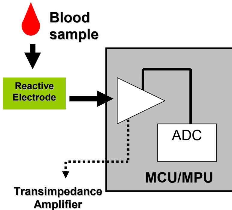
*Fig 2. Test strip basic block diagram*
