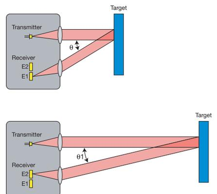
Figure 3. Principle of Background Suppression
