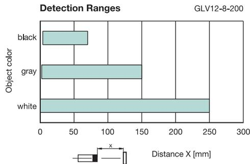
Figure 1. Effect of Color on Diffused Sensing
