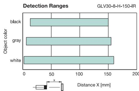
Figure 2. Effect of Color on Background Suppression Sensing
