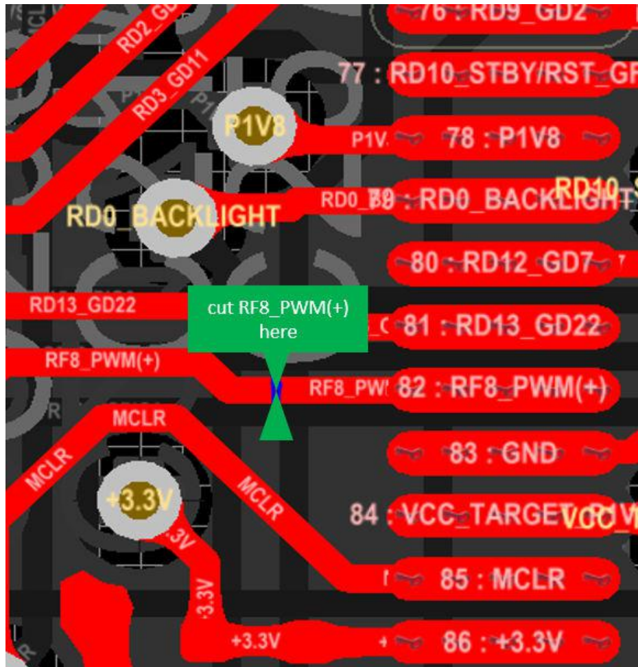
Figure 3. Cut location for RF8_PWM(+) trace
