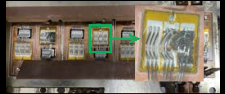
Figure 1 Image of failed IGBT-die with molten top metallization
