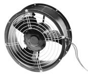
The tube-axial fan is the most common type used in electronic cooling systems. It is similar to a propeller fan except for a venturi tube placed around the propeller to reduce vortices. Tube-axial fans, typically used for general hot air removal as well as heat transfer from specific hot spots, often have ball bearings to provide long life. The vane-axial fan has vanes that trail behind the propeller in the airflow to straighten the swirling flow of accelerated air.
