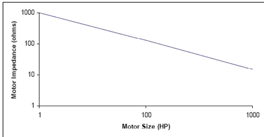
Figure 2. Motor impedance relative to motor size
