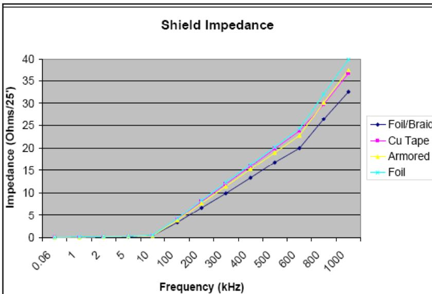
Figure 4. Shield/Ground impedance of the various cable types
