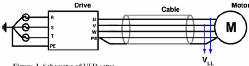
Figure 1. Schematic of VFD setup
