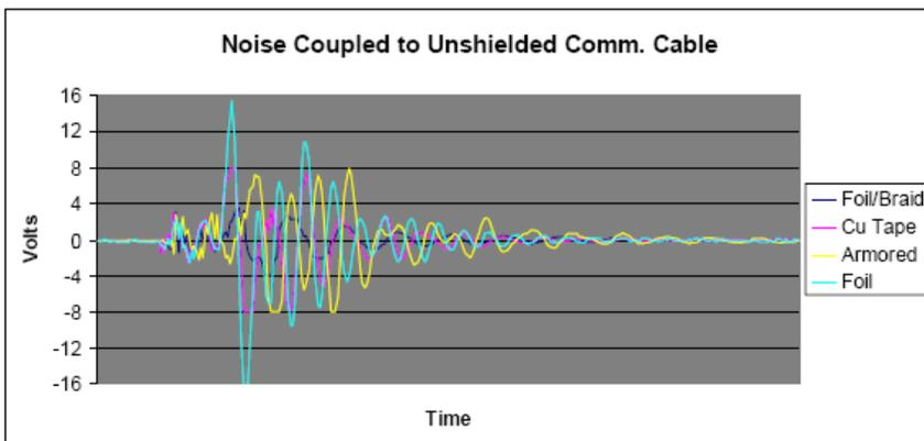
Figure 3. Noise coupled from VFD cables to unshielded instrumentation cable
