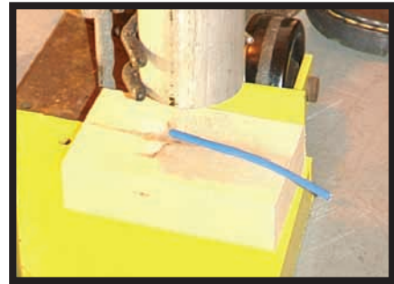
In the cold impact test, after the cable is cooled an aluminum weight smashes against it.
