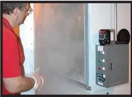
In the cold bend test, the cables were first placed into a cold box.
