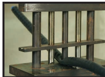
A chisel-point mandrel on an Instron machine performs the cut-through procedure.
