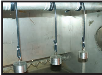
Then they were partially wound around a mandrel and subjected to the tension experienced through the use of an aluminum weight.
