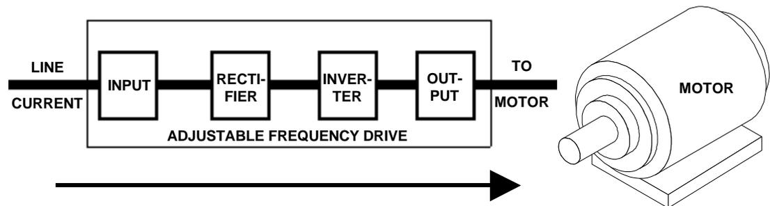
FIGURE 3. CURRENT PATH FROM LINE TO MOTOR
