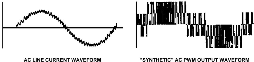
FIGURE 4. LINE CURRENT VS. SYNTHETIC AC CURRENT SINE WAVES
