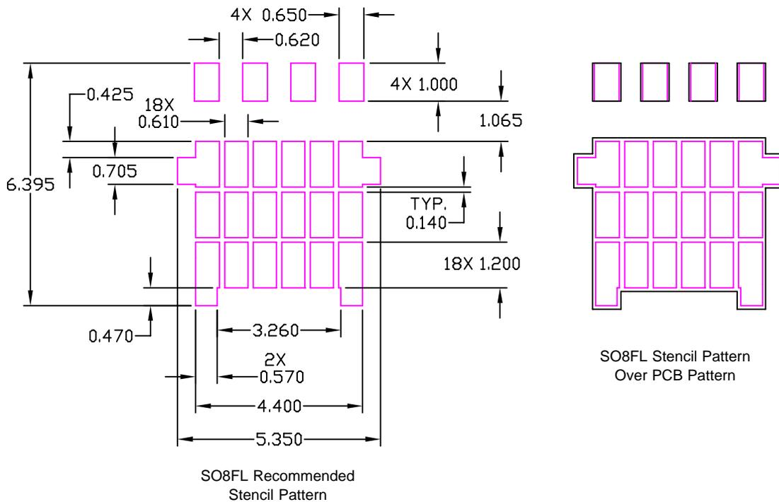
Figure 5. Solder stencil design illustrating how stencil openings are divided into an array for large die pads.
