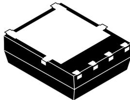
Figure 1. The Underside of an SO8FL Package
