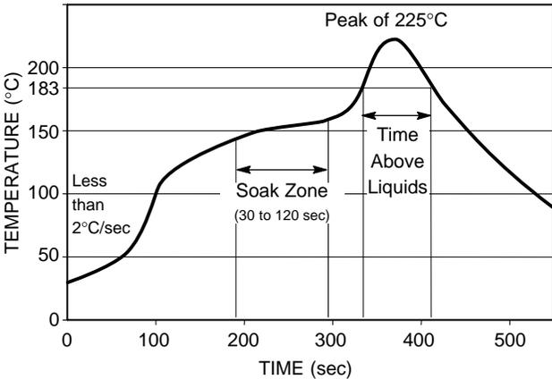
**Figure 6. Typical Reflow Profile for Standard Tin/Lead Solder**
