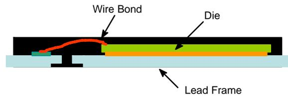
Figure 2. Cross-Section of SO8FL Package
