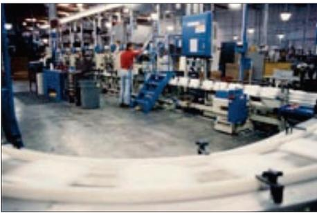
Most motors, lighting and indicators can tolerate sags of short duration with negligible detriment to production (perhaps a fan slows down briefly or a light flickers, but production goes on). The most sag-sensitive, and usually most critical, component is the AC/DC power supply used to power all DC control and logic circuits.
