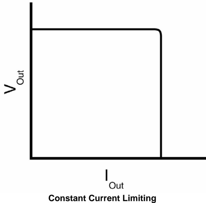
**Current Limit Shutdown:** In some power supply designs, when an overload occurs the power supply will begin to go into a constant-current limit mode, but when the output reaches a preset reduced voltage, the supply will shutdown. Recovery from this condition can be automatic or require recycling of the input power.
