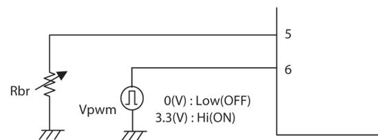
some applications, this input can be connected to a temperature sensing device that could reduce the current flow through the LEDs as the temperature rises, thus providing a means for temperature compensation. The “Vpwm” is a Pulse-Width-Modulation input that controls the LED brightness by varying the duty-cycle of the input signal from 1 percent to 100 percent. Typical PWM frequencies can range from 180 Hz to 270 Hz.
