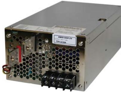
**Above is a photo of an HWS series power supply that can provide 1000 watts of output power and features alarm signals and active current sharing. Two or more of these supplies can be connected in parallel with external “ORing” diodes to form a redundant and fault tolerant power system.**
