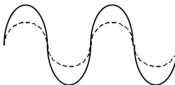
**Figure 2. Voltage and Current waveforms are sinusoidal and in-phase; PF=1.**
