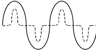
Figure 3. Voltage waveform is sinusoidal, current waveform is non-sinusoidal but in-phase;  $PF < 1$ .
