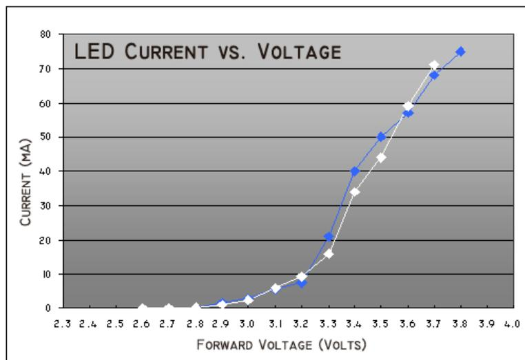
In viewing the white curve above, it's important to notice that the forward voltage drop across the LED between 3.2V and 3.6V (a 0.4V change), results in a current increase of over five times (from 10mA to 60mA). In this example, if the maximum allowable LED current is 40mA and if 60mA or more current is allowed to flow through it, the LED could be destroyed or its operational life substantially reduced.
