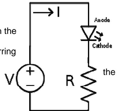
$$R = (V_s - V_d) \div I, \text{ therefore, } R = (5V - 2V) \div 0.02A = 150 \text{ ohms}$$
