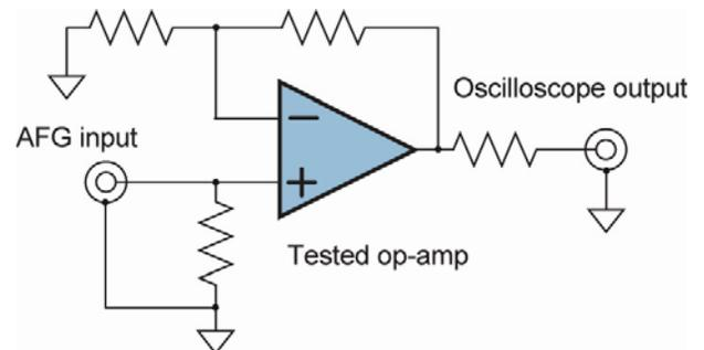
**Figure 1: Slew rate measuring circuit.**
