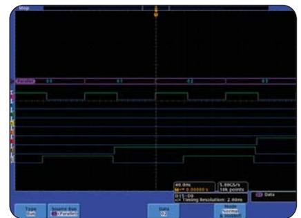
► Clocked parallel bus display, decoding a 7 bit counter.
