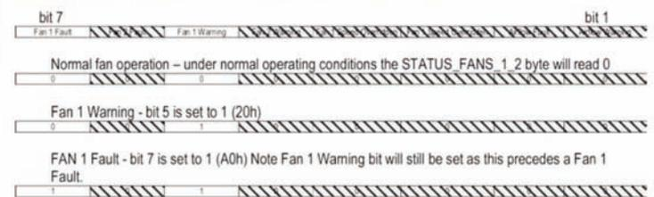
Figure 3 – Status fans fault indication
