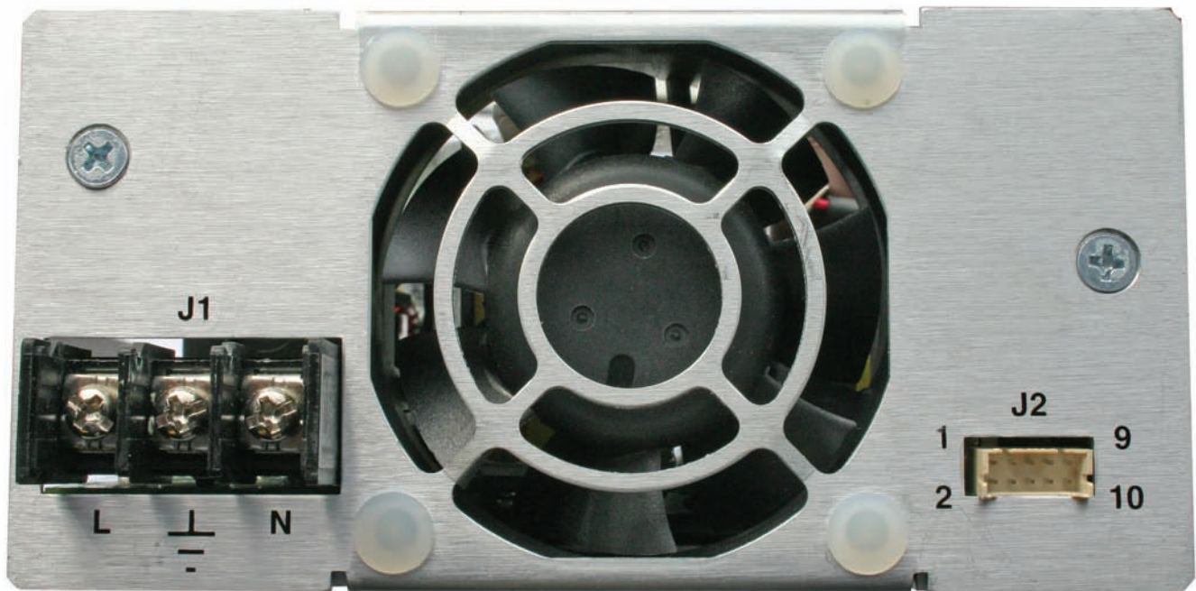
Figure 4. Finger guard has been pressed outwards slightly to reduce noise.
