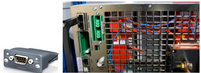
Figure 6. Anybus communication interface modules (on the left) are easily installed into an EA power supply's digital interface slot (on the right) and can be swapped based on changing test needs with a simple screwdriver.
