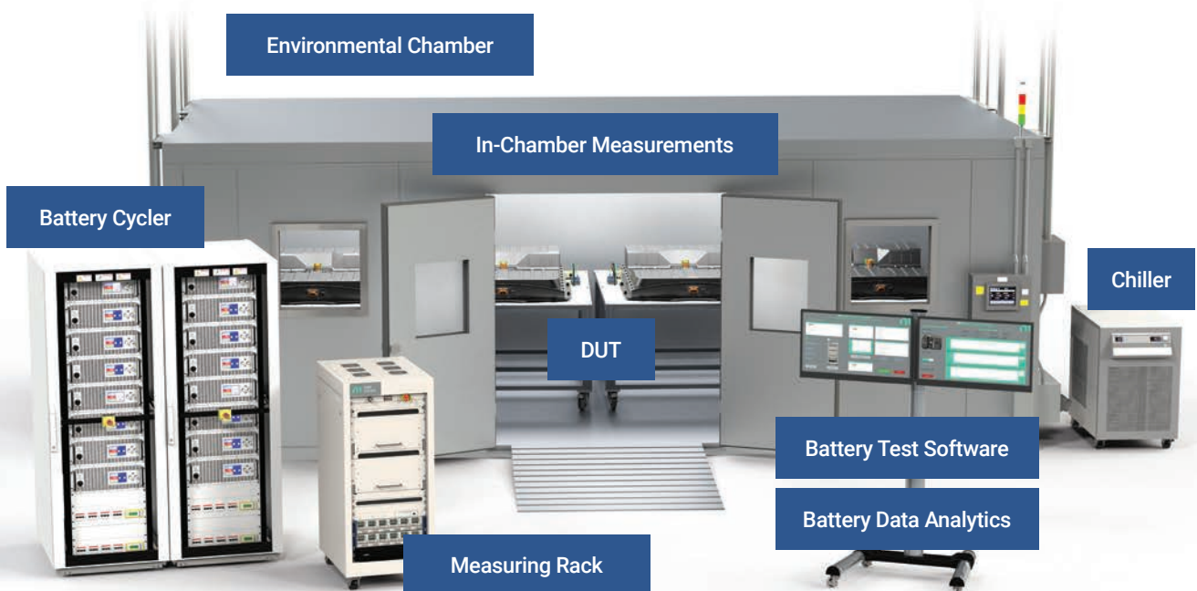
Figure 2. Typical lab setup for battery validation.
