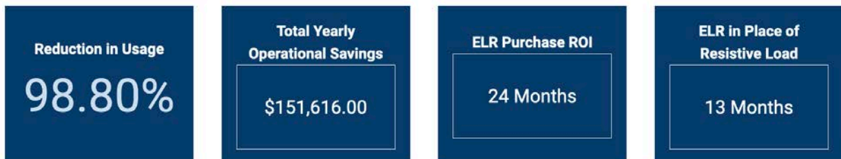
Figure 7. The annual ROI for an EA bidirectional power supply for a 20 kW load with a 40-hour work week.
