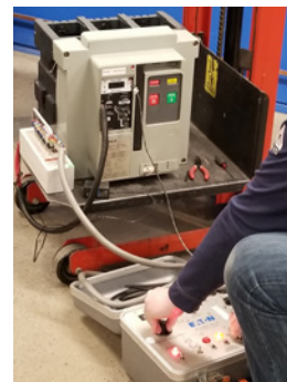
Secondary Injection Testing
