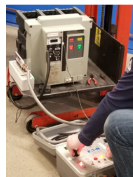
Secondary Injection Testing
