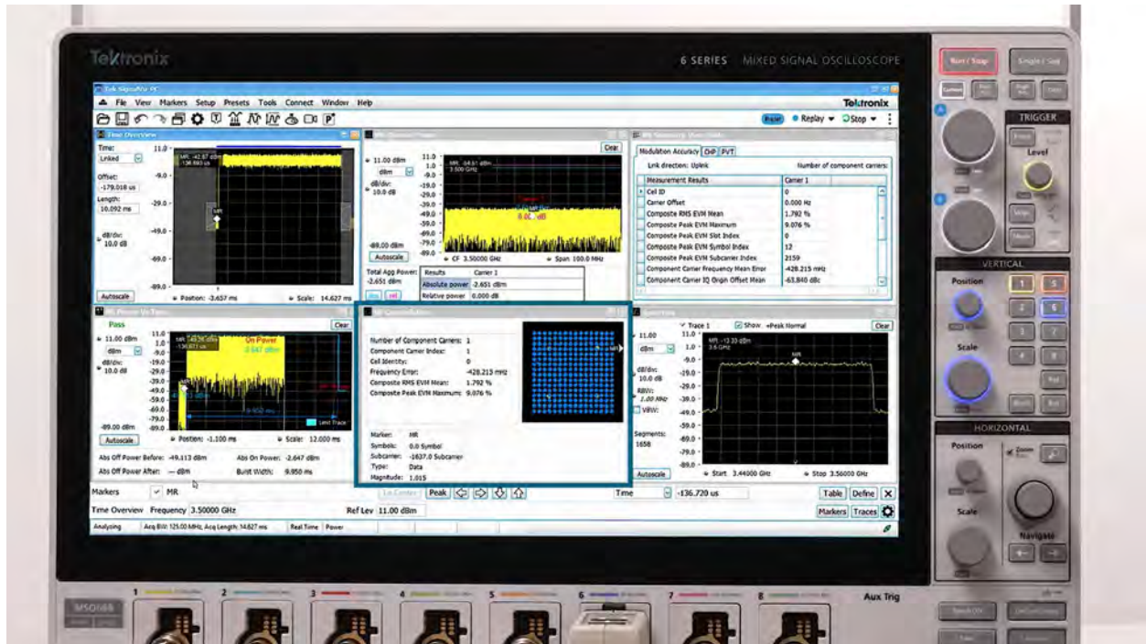
Figure 4. In this measurement the EVM is higher than expected.
