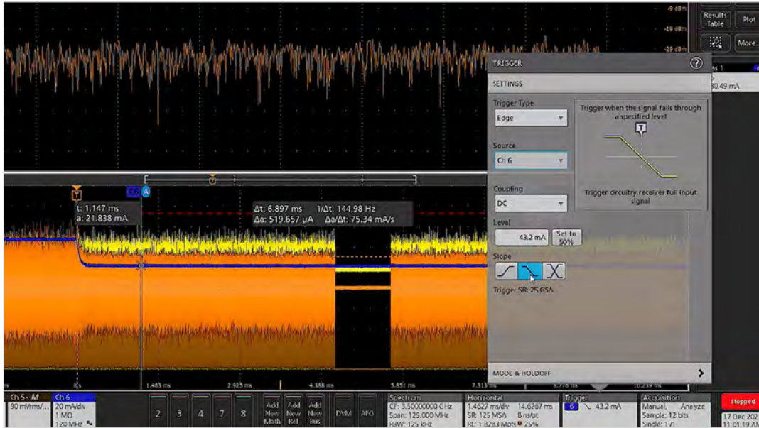
Figure 7. The trigger is set to capture on a decrease in current, to consistently acquire the undercurrent condition.
