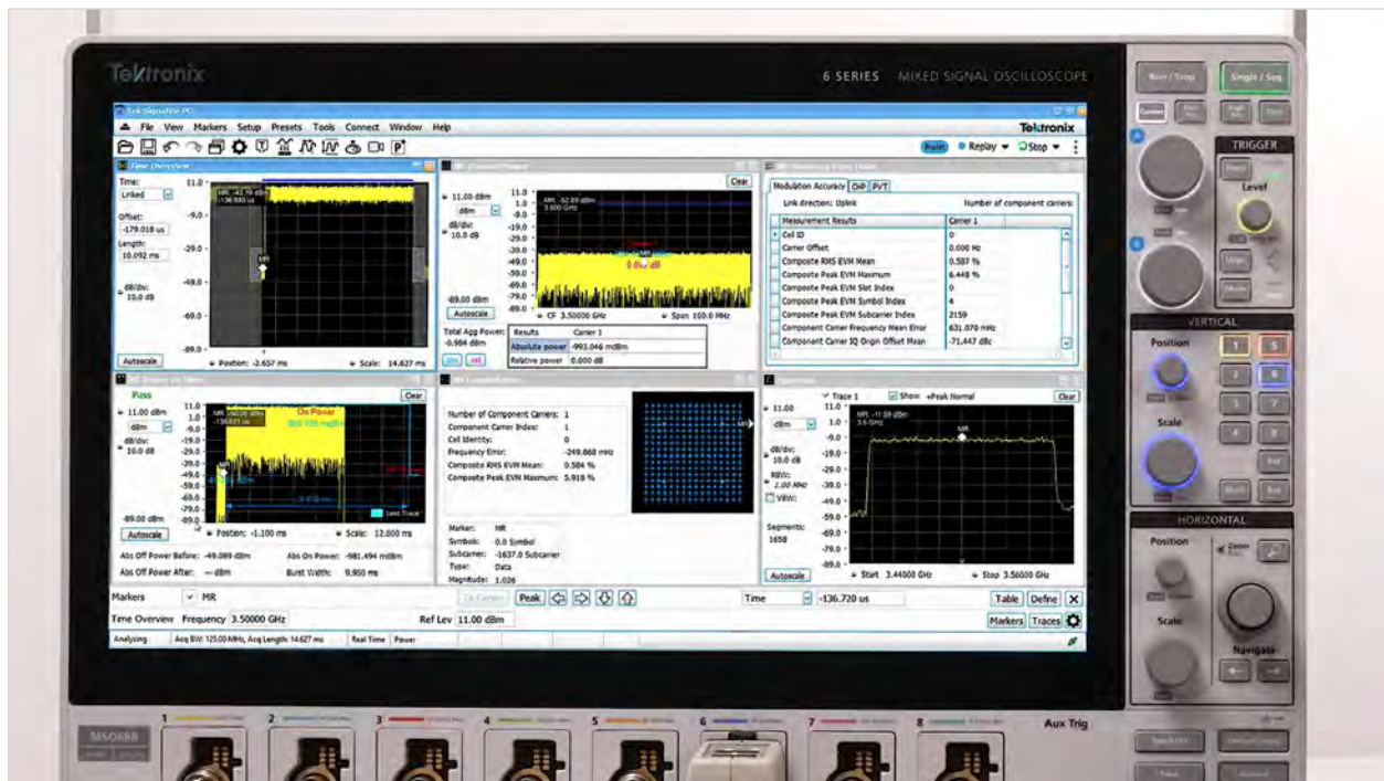
Figure 3. In this measurement the EVM shown in the constellation display is as expected.
