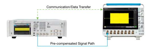
The simple example shown here illustrates how the application of pre-compensation can flatten the RF amplitude of a 1 GHz wide Linear Frequency Modulated (LFM) pulse that is centered at 5 GHz.
