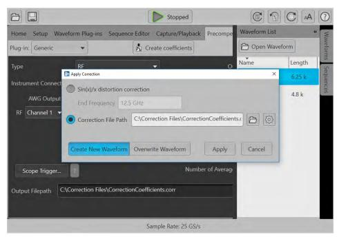
When you select the coefficients, a dialog box will show up to show you the filter's characteristics that the AWG will apply to the waveform:
