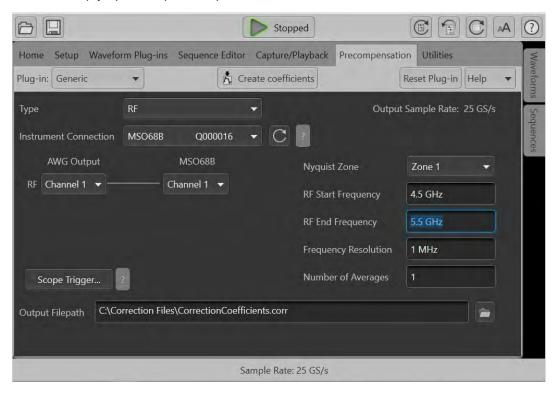
This plug-in generates a test signal which is measured on the oscilloscope, and it uses that measured result to generate the filter. The first thing to do is tell the AWG to "connect" to the oscilloscope by providing its IP address. This is most often done through Ethernet using VISA. As long as the VISA server on the AWG can "see" the scope, it will show up on the drop-down "Instrument Connection" list.
