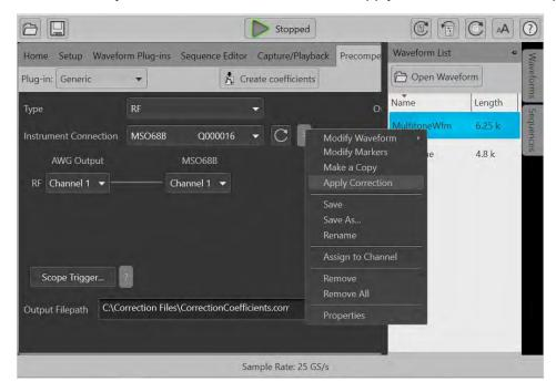
Select the "Correction File Path" radio button, and use the folder icon to navigate to the correction filter file you just created. Select the "Create New Waveform" button, and hit APPLY to create a precompensated version of your original waveform.
