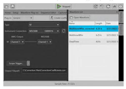
Drag the waveform into the channel (Ch1, in this example) to load it and get it ready for playback. Click on the "play" button to generate the pre-compensated waveform.
