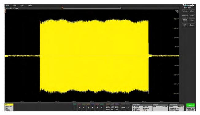
We can observe a fair amount of ripple and some droop in the RF envelope, resulting from the RF cable and the AWG's output.
