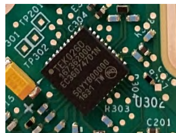
Figure 4c: New Tektronix analog front end ASIC (TEK026D)
