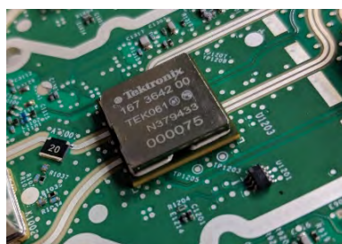
Figure 4b: New Tektronix analog amplifier ASIC (TEK061)
