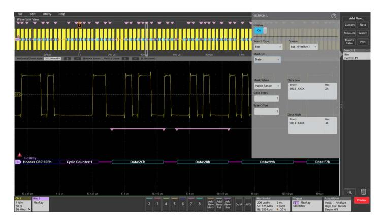
But how many of the events occurred? To find all of the bus events that meet a specific search criteria, you can use automated Wave Inspector search. The setup is similar to the bus trigger setup, allowing the oscilloscope to find and mark all of the specified bus events.
