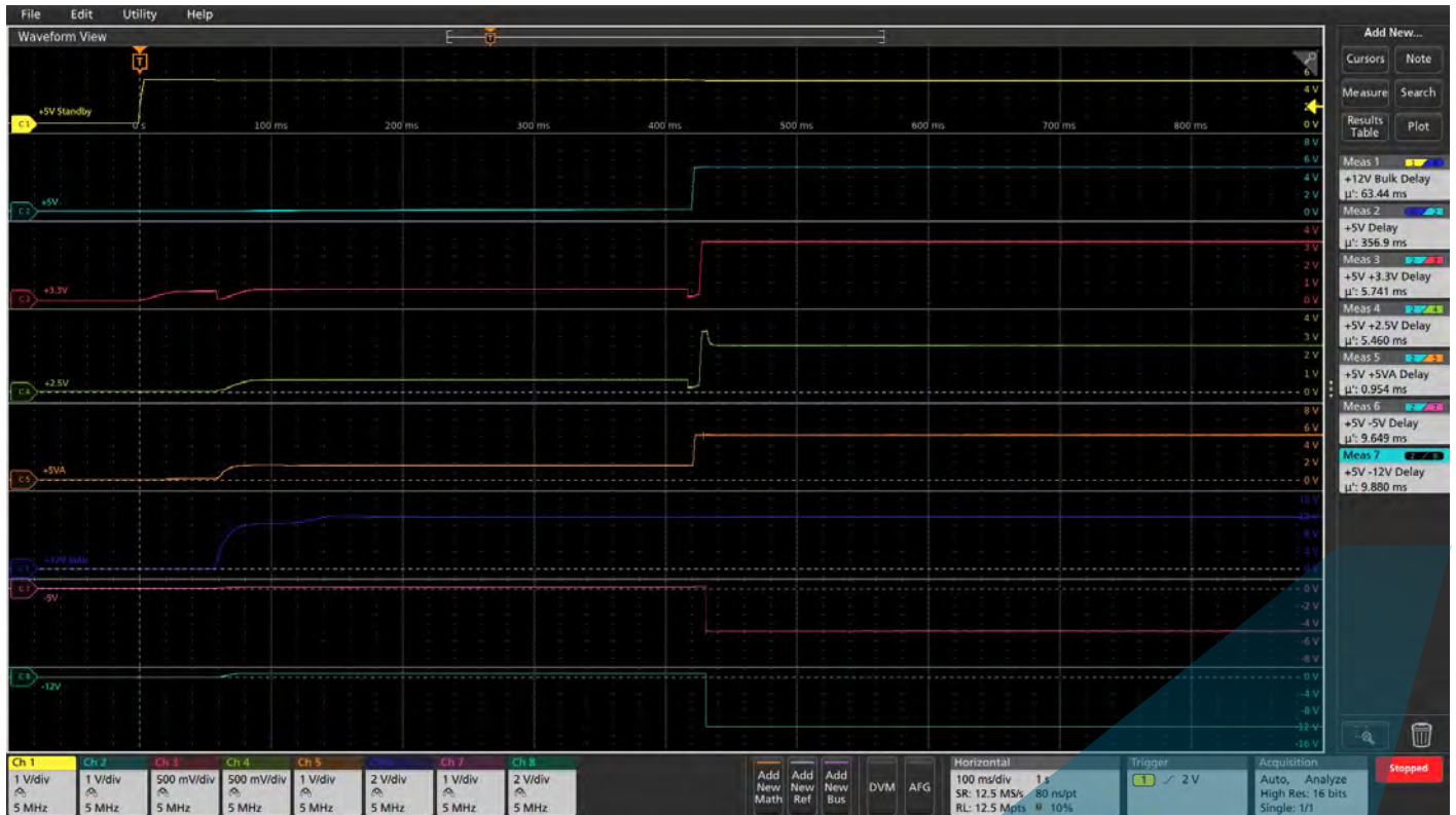
Turn-on timing of seven of the regulated power supplies in the product
