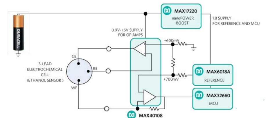
Figure 3: Block diagram of battery-powered electrochemical sensing system with 1V op-amp
