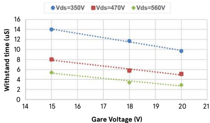
**Figure 3: Short Circuit Withstand Time of MSC035SMA070B.**
