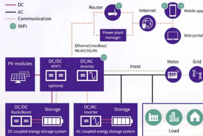
**Figure 2: An example residential solar power installation with battery storage, EV integration and utility energy feed-in.**
