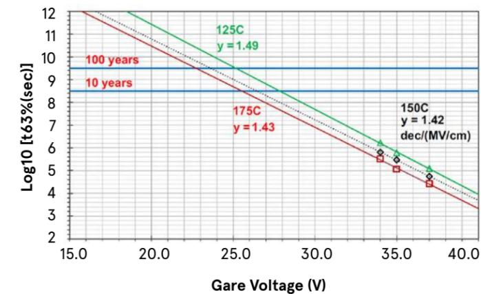
**Figure 4: Projected Device Lifetime Under Different Gate Voltage.**
