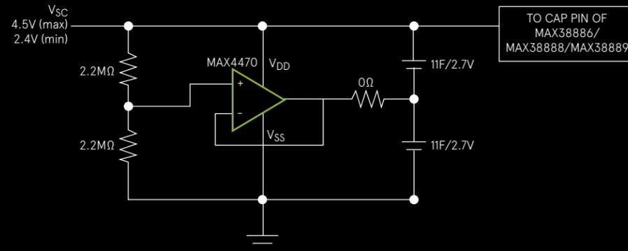
Figure 3. Voltage balancing using an op amp circuit.
