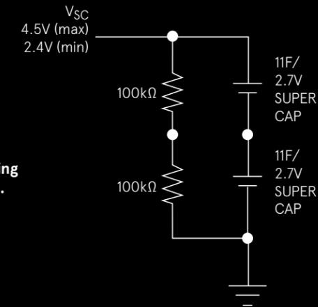
Figure 2. Voltage balancing using balancing resistors.
