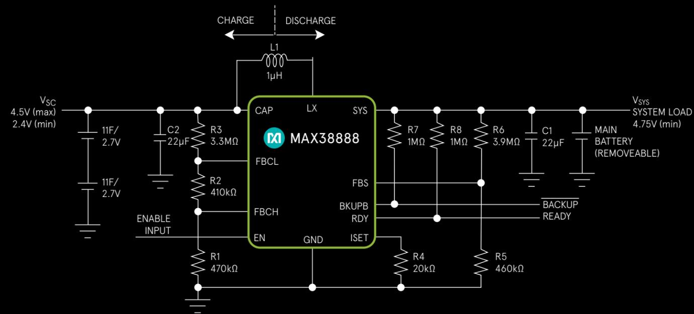
Figure 1. Application circuit of MAX38888
