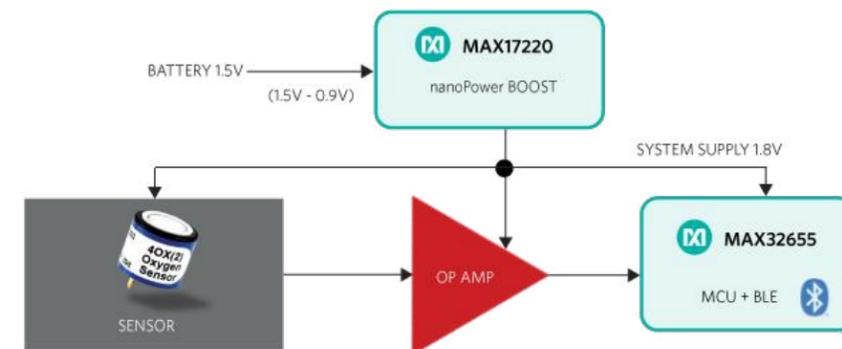
Figure 2: Traditional architecture of battery-powered sensor system
