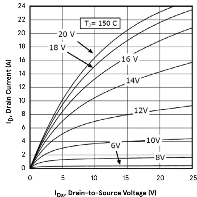
**Figure 2: I-V Curve of MSC360SMA120B Under Different Driving Voltages at T<sub>j</sub> = 150°C.**
