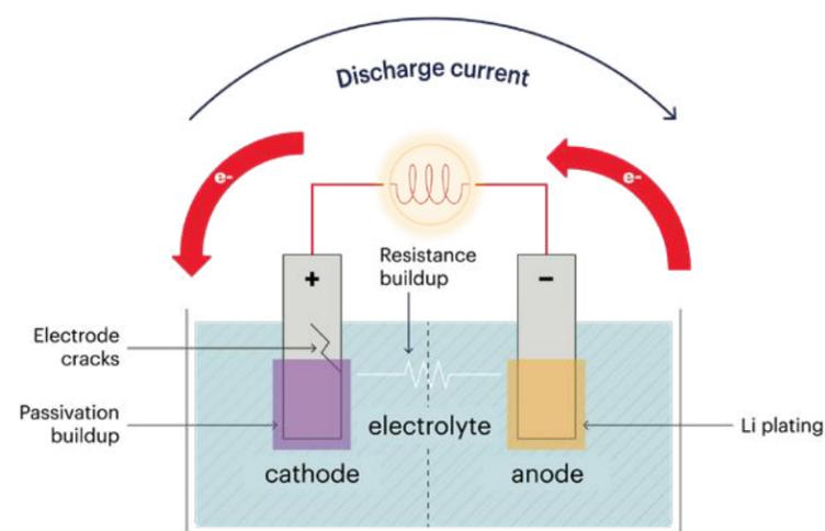
Figure 2. Internal battery failure mechanisms over time.
