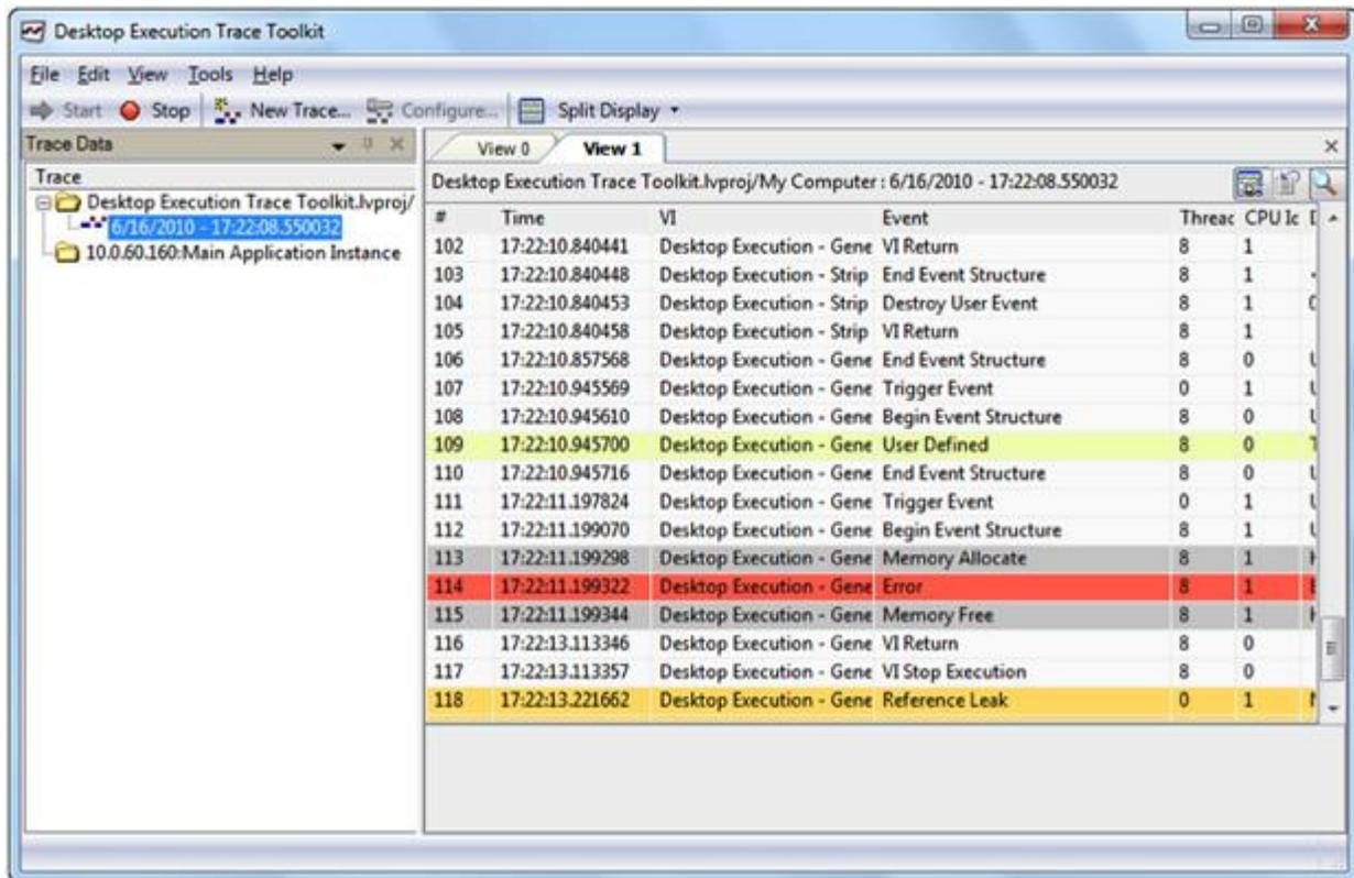
**Figure 12.** If you need lower-level debugging, you can use the LabVIEW Desktop Execution Trace Toolkit to view the dynamic execution characteristics of an application.
