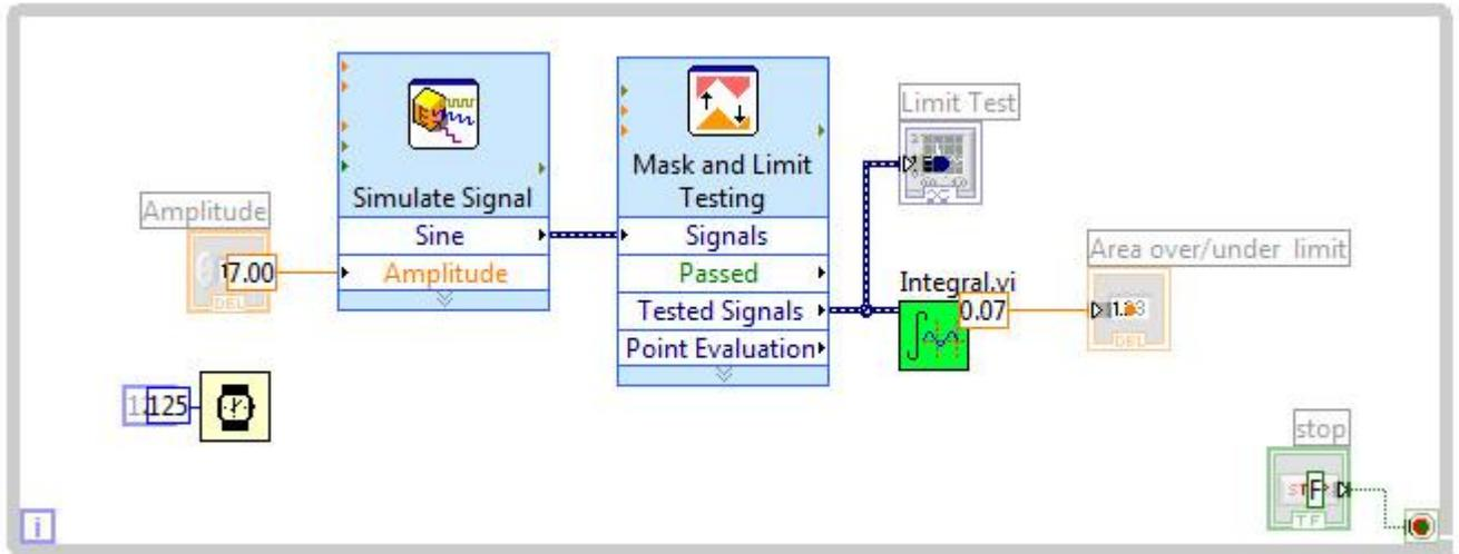
**Figure 3. Highlight execution provides an intuitive way to understand the execution order of G code.**
