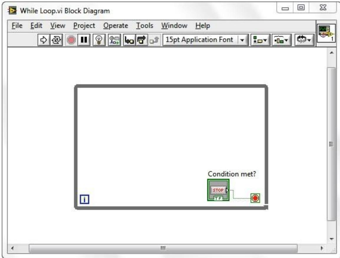
**Figure 1. A While Loop in G is intuitively represented by a graphical loop, which executes until a stop condition is met.**
